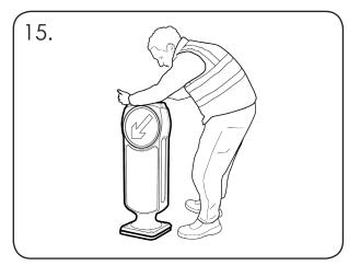
To test, cover the solar panel and Light Dependent Resistor [top of the bollard] for approximately 10 seconds. The sign face should illuminate.
